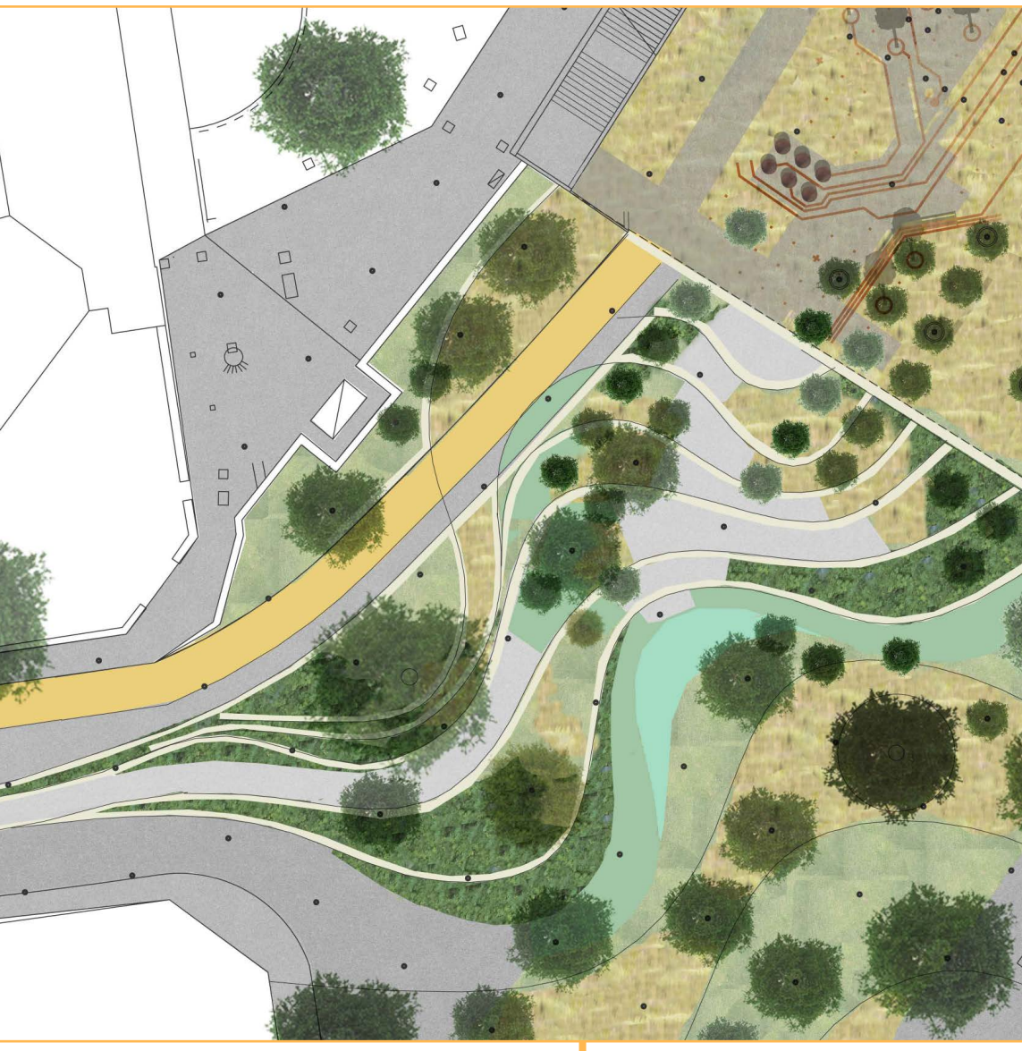
Slope plan Terraced landscapes to create play space, informal seating and shallower access routes; Cycle route marked with vehicle access maintained for servicing park; Gabion walls formed using recycled material from park construction process.
